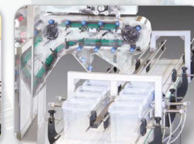
PLC controlled device for counting & filling lollipops into containers.
